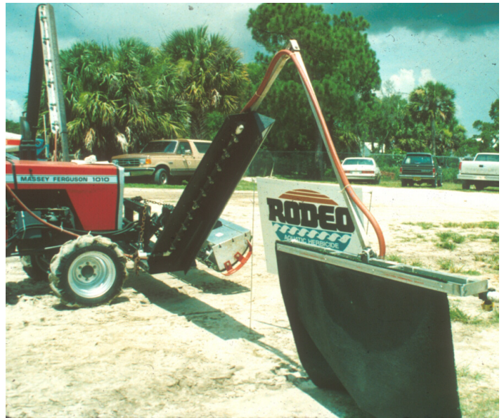
Figure 8. Wiper used to apply aquatic herbicides to grove ditches. Credits: J. Hebb
