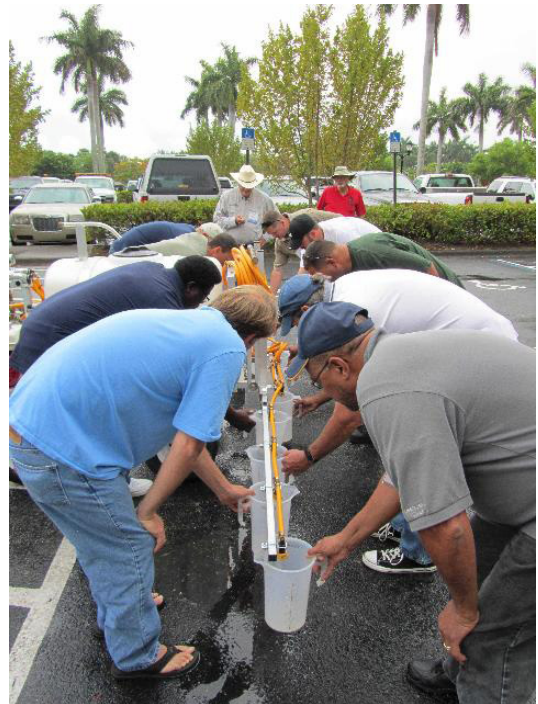
Figure 1. Checking nozzle output. Credits: UF/IFAS Pesticide Information Office
