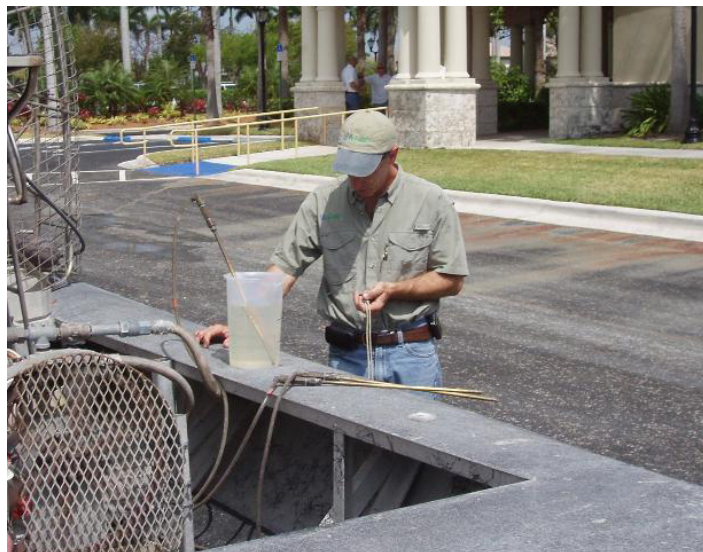
Figure 10. Measuring herbicide withdrawal of a direct metering system.
