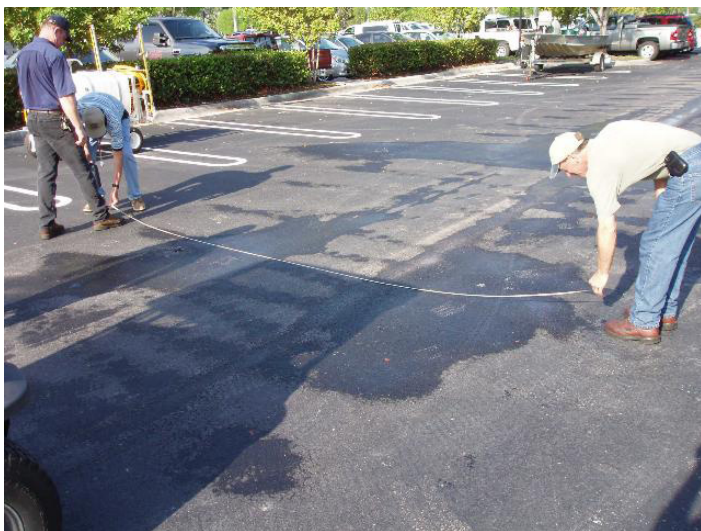
Figure 9. Checking swath width of a sprayer gun on asphalt.
