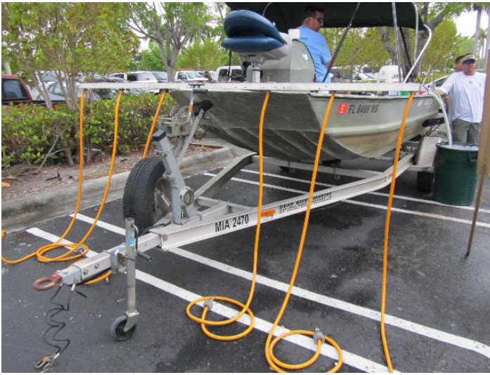
Figure 5. Drop hoses for subsurface application. Credits: UF/IFAS Pesticide Information Office
