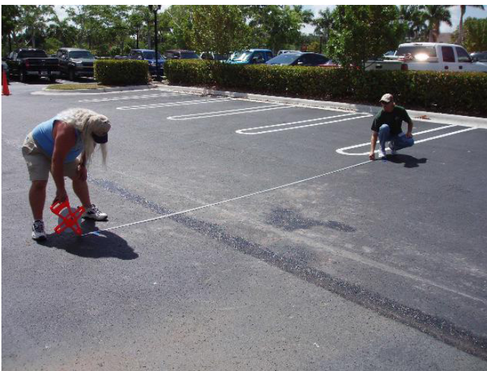
Figure 13. Measuring the swath width of a granular spreader. Credits: UF/IFAS Pesticide Information Office
