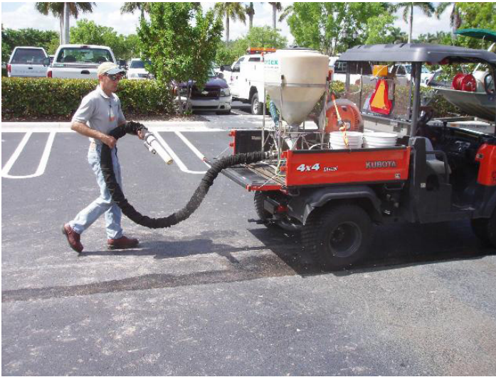
Figure 12. Granular spreader with handheld gun. Credits: UF/IFAS Pesticide Information Office
