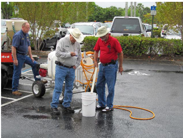
Figure 8. Measuring output of a handheld sprayer gun.
