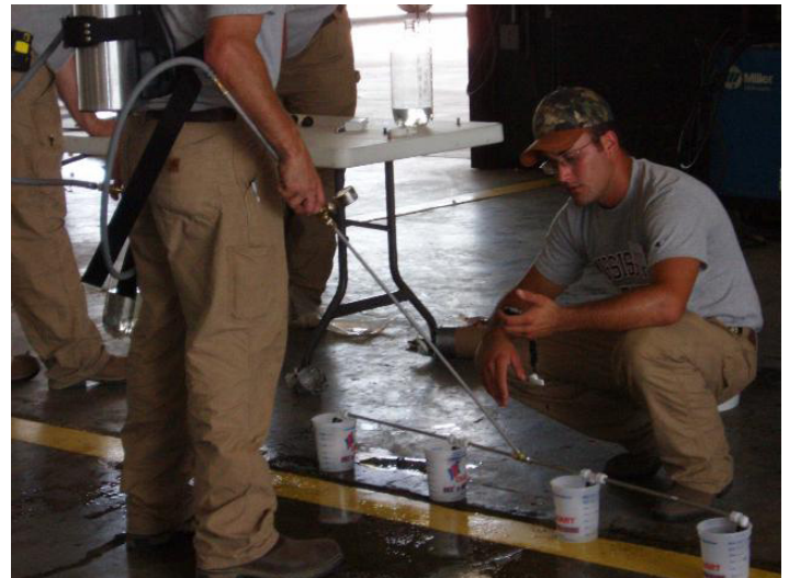
Figure 4. A nozzle uniformity check from a backpack sprayer. Credits: UF/IFAS Pesticide Information Office
