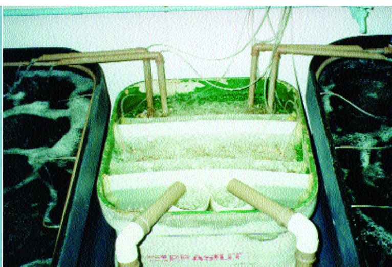
Figure 31 Close-up of a biological filter shared between two larval tanks in Brazil, showing the water entering the mechanical filters (foreground), from where it passes through the biological filter and exits back to the two tanks by means of simple airlift pumps
