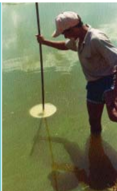
Figure 78 Measuring transparency can be very simple, even when the design of the Secchi disk is unconventional (Peru)
