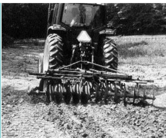
Figure 66 The bottoms of ponds can be tilled with a disc harrow (USA)
