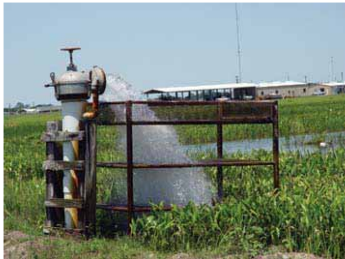
Figure 7.3. Aeration screens can be designed not only to aerate, but also to reduce the transfer of wild fish into ponds during pumping.
