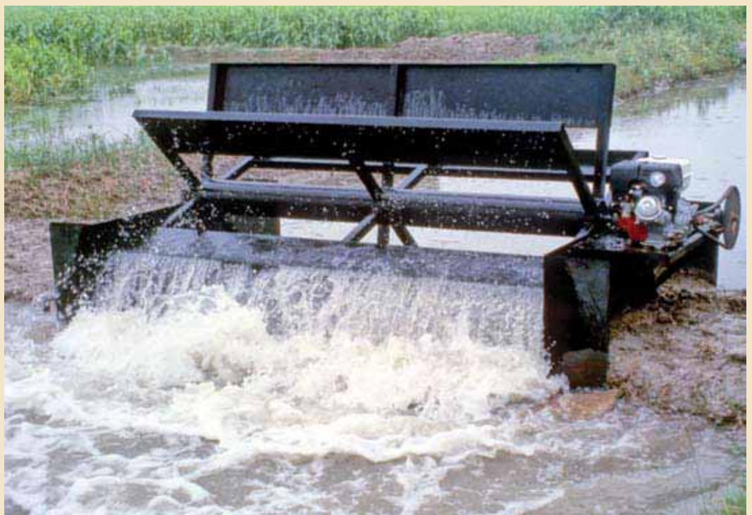
Figure 4.4. When ponds are extremely level, recirculation can be accomplished using commercially available or shop-built paddlewheel aerators.
