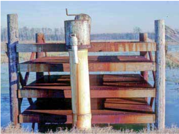
Figure 7.8. Well water often contains iron in the reduced (un-oxidized) form. This problem can be corrected by sufficient aeration.
