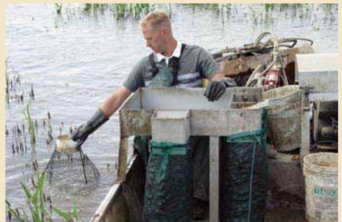
Figure 8.8. Typical shop-built "in-boat" grader designed to allow submarketable crawfish to be returned to the pond immediately after harvest via a chute placed below the parallel bars.
