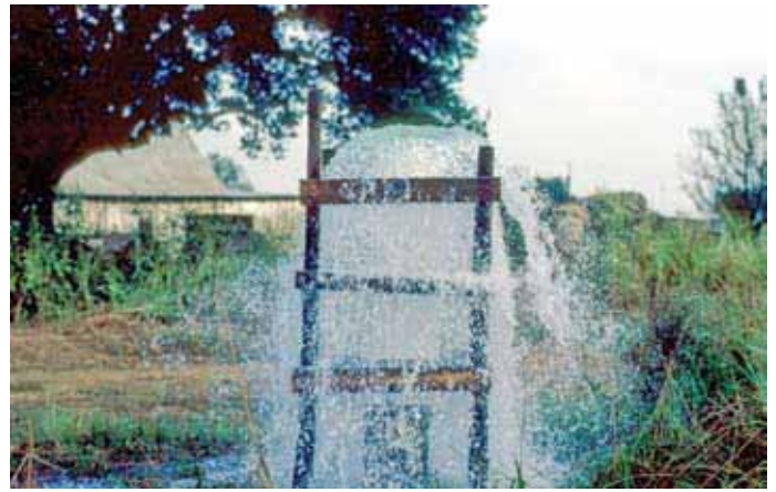
Figure 7.7. The key to good aeration during pumping is to maximize contact between air and water.
