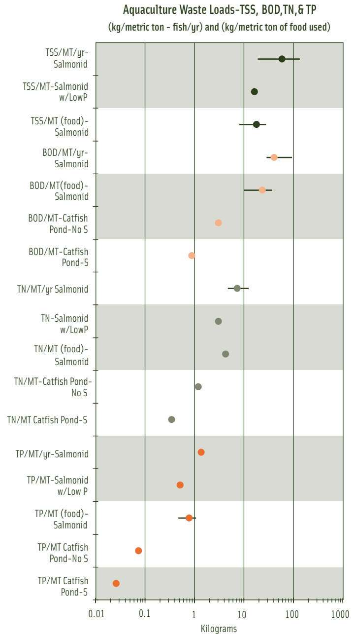
Figure 11. Waste loads of various representative aquaculture operations. total suspended solids (TSS) (●), biochemical oxygen demand (BOD) (●), total nitrogen (TN) (●), or total phosphorus (TP) (●) discharged per metric ton (MT) of fish production or per metric ton of food used. Salmonid values based on cited references in Beveridge et al. (1991) or Axler et al. (1997). Catfish values based on Tucker (1998) and Tucker and Hargreaves (1998) reported discharges in kg/ha from ponds with and without storage (S), assuming a production of 5,000 kg/ha.
