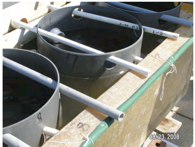
Figure 1. A typical upweller silo in use.
