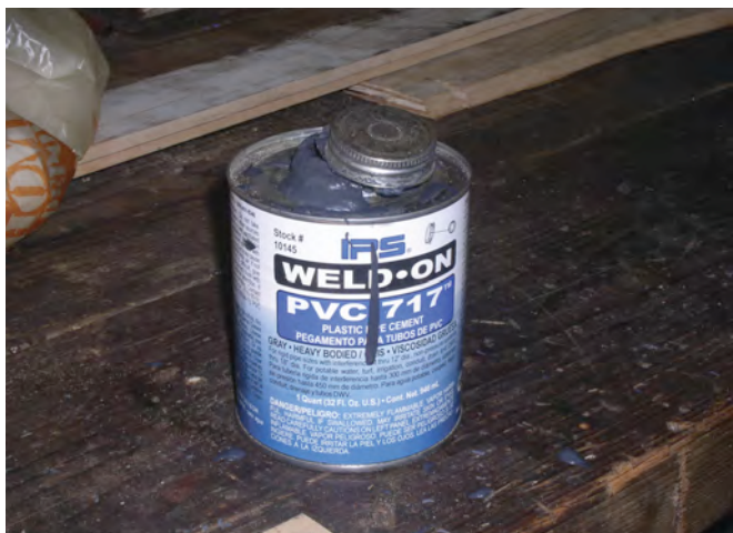
Figure 14. Thick PVC glue works best.
