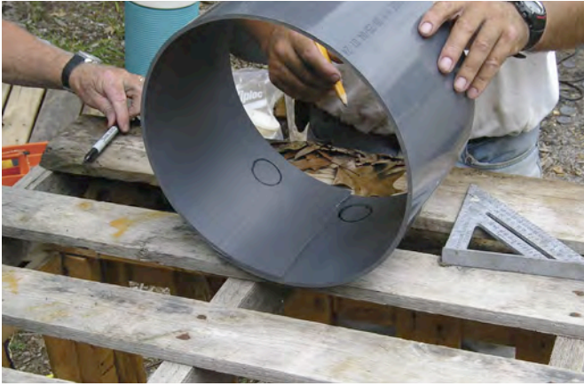
Figure 8. The jig for placing support holes and the connector hole on the silo.
