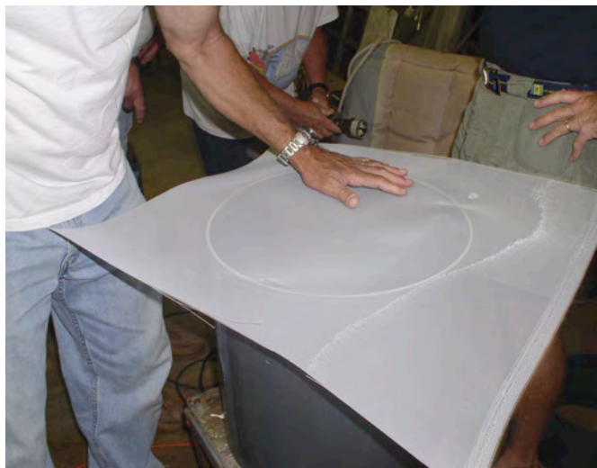
Figure 11. Laying the mesh onto the silo before clamping.
