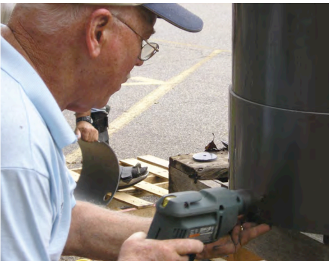
Figure 9. Using the jig to position the holes on the sides of the silo.
