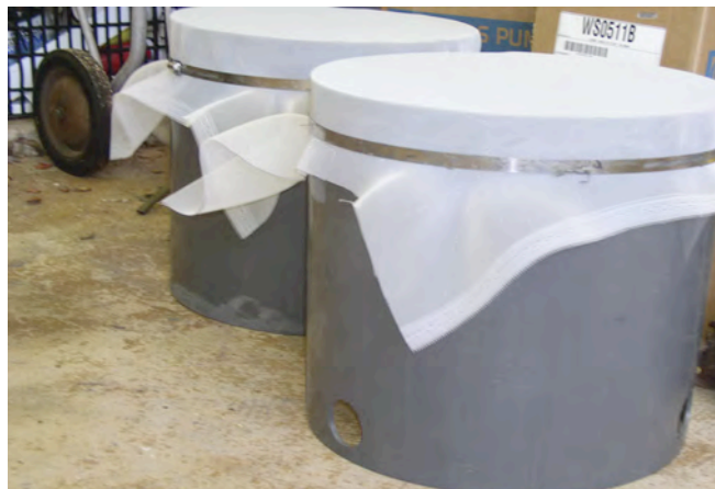
Figure 12, Hose clamps hold the mesh for the next step, gluing on the ring.
