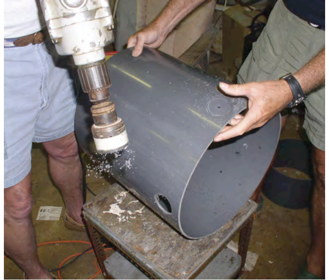
Figure 10. Using the hole saw to cut out the support holes and the connector hole.
