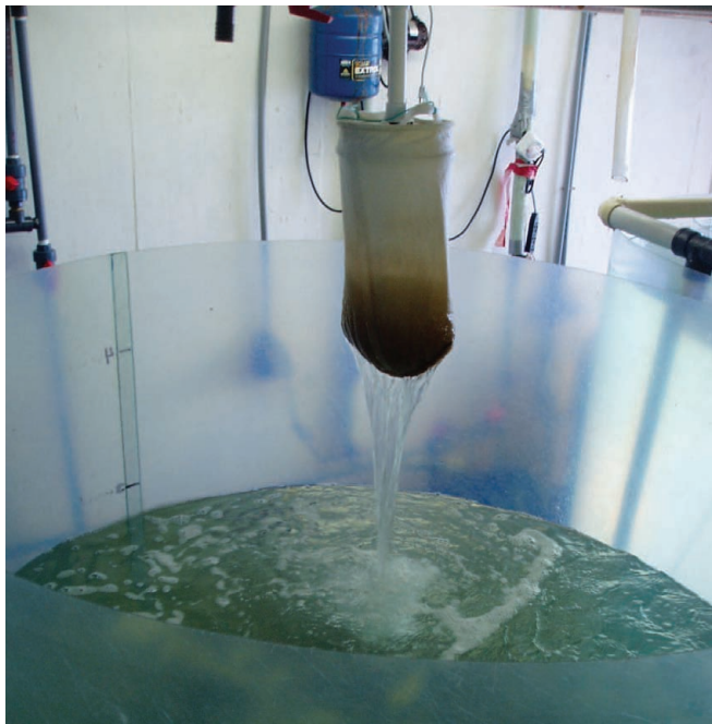
Figure 2. Culture water is filtered through a bag filter.
