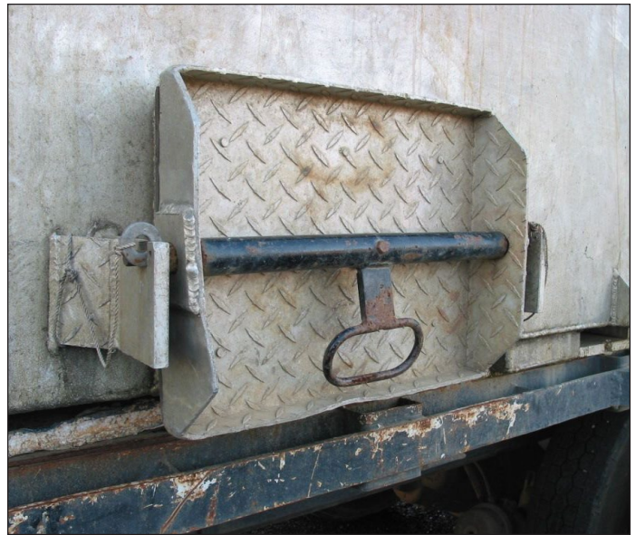
Figure 3. Rectangular steel dump gate on aluminum tank.
