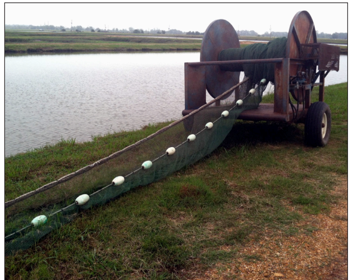
Figure 11. Drying and exposure to sunlight will help reduce pathogen loads on large pieces of equipment, such as this seine net. Photo credit: Matt Griffin, NWAC, Mississippi State University
