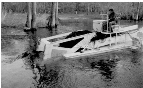
Figure 8. Aquatic plant harvester clears weeds from a lake surface.
