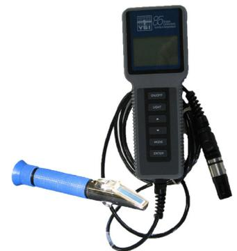
Figure 3. A refractometer is a relatively inexpensive instrument for checking salinity. Digital salinity meters are more costly but can be more precise. Different models can also measure other water quality characteristics. Photo: Jill Christoferson
