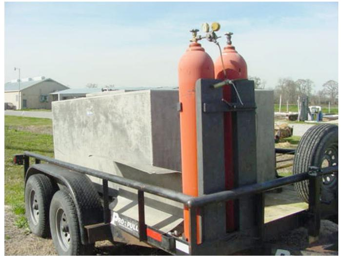
Figure 1. Oxygen cylinders and hauling tank on trailer ready for transport. Photo: Greg Lutz
