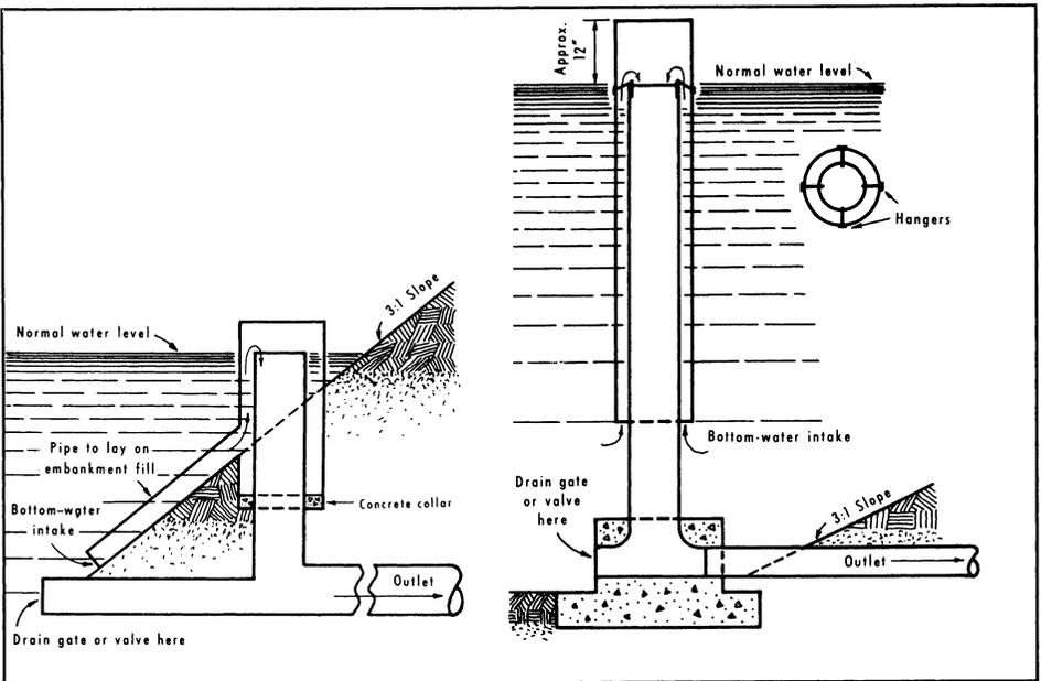
Figure 2. Examples of trickle tubes that allow the automatic removal of poor-quality bottom water during the summer.
