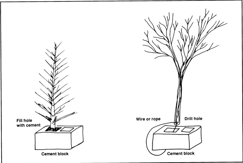
*Figure 4. Fish attractors constructed from trees and cement blocks.*
