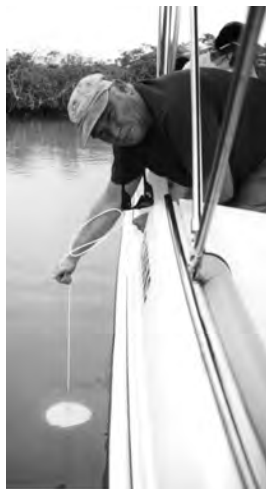
LAKEWATCH uses solid white Secchi discs, as shown here.
