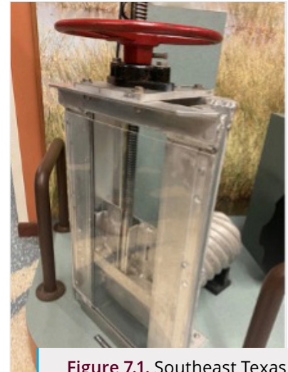
Figure 7.1. Southeast Texas water gate system to control water flow and levels. Photo: Nikki Fitzgerald
