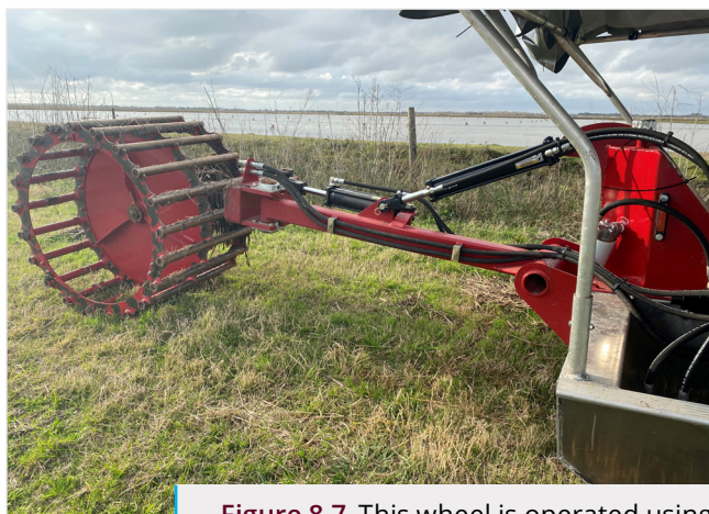
Figure 8.7. This wheel is operated using foot pedals and leaves the driver's hands free to empty and rebait the traps.
