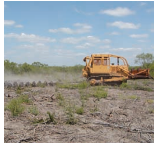
Figure 20. Mechanical treatments are often used to reduce brush cover and structure. Mechanical methods kill the tops of plants, but many brush species vigorously re-sprout from the roots. Prescribed burning or spot treatments with herbicide can lengthen the life of the original treatment.
