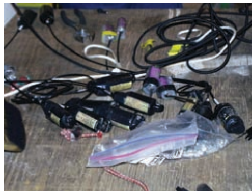
Figure 7. A radiotransmitter is about the size of D cell battery (about 3 to 4 ounces) and is attached to a 14-inch antenna. Radiotransmitters send specific radio signals for tracking individual turkeys.
